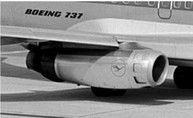
Left: Placement of the engines on the Boeing 737 classic
